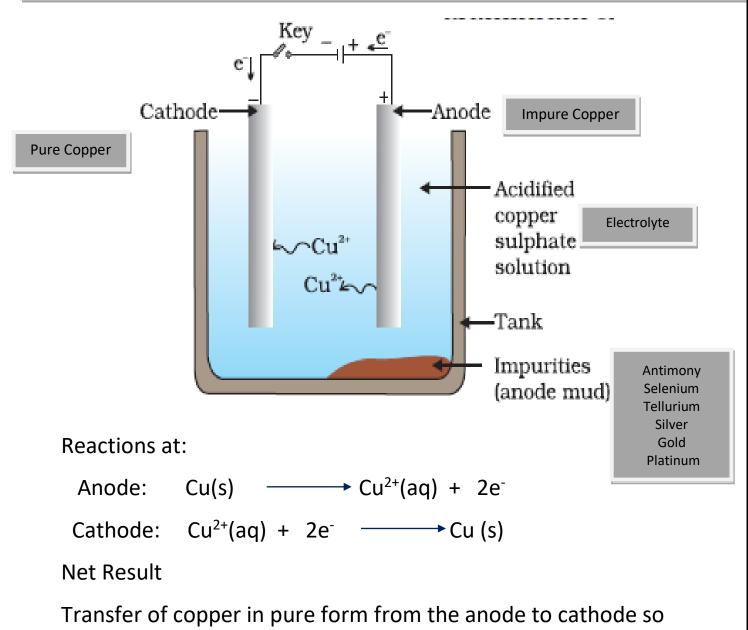
pure copper deposited on the cathode.
